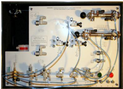
10. <u>Fully automatic circuit using a 5/2 Solenoid control valve, a Single and a Double acting actuator. Control is achieved using a feedback signal to the PIC Logicator interface board and Software.</u>
