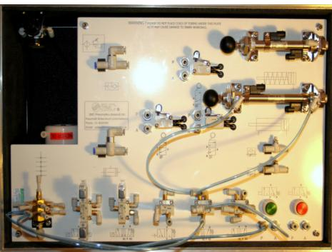
6. <u>Double acting actuator speed control using a 3/2 pushbutton valve, a 5/2 Pilot controlled pneumatic valve and two flow control valves.</u>
