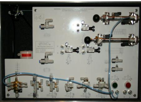
4. Actuator speed control using a 3/2 Pushbutton valve with a single acting actuator and flow control valve.
