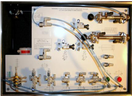
8. The AND circuit using two 3/2 pushbutton valves, a two pressure valve and a single acting actuator.
